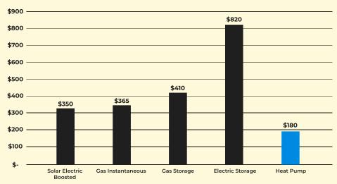
Data sourced from Sustainability Victoria's Hot Water Running Costs 2020 and compares running costs of a 5.5-star gas storage system, 7-star gas instantaneous system, electric storage off-peak system, high-efficiency solar gas boosted system, high-efficiency solar electric boosted system, high-efficiency hot water heat pump on off-peak tariff.
