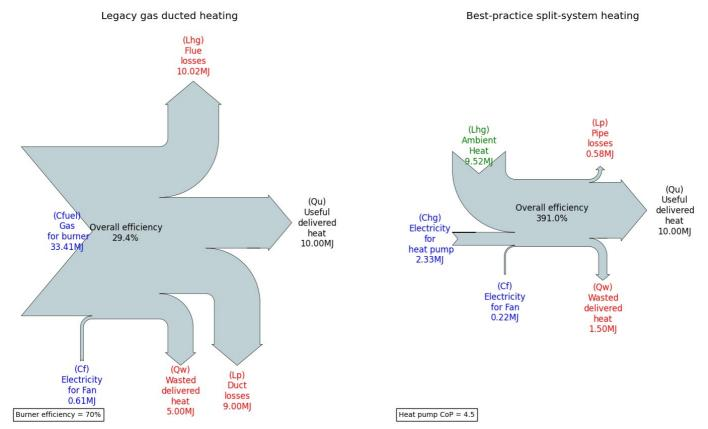
Space heating relative efficiency: gas ducted *vs* split system heat pump.
